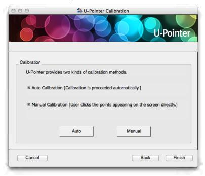
Auto calibration\*: click "Auto" and the calibration process will run automatically.
