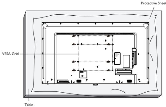
1. Lay a protective sheet on a table, which was wrapped around the display when it was packaged, beneath the screen surface so as not to scratch the screen face.
