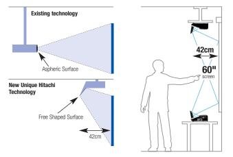
• **Ultra Short Throw** – Using Hitachi's new unique high performance lens. We are able to dramatically reduce the throw distance, combined with the introduction of a high angle projection capability, the quiet ED-A111 projector can be sited only 42cm away for a 60" screen.
