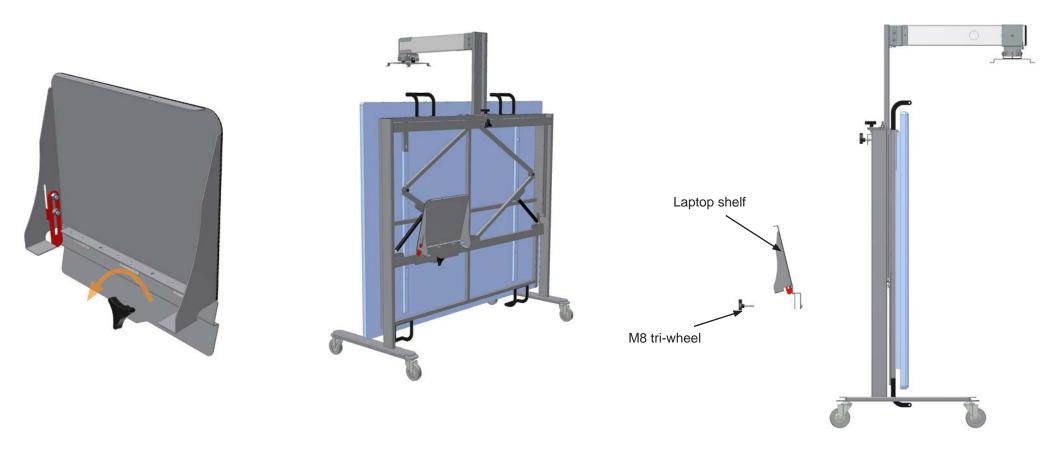
22 - Undo the tri-wheel from the laptop shelf. Hook laptop shelf onto support beam. Re-attach tri-wheel. Slide the shelf to the desired position before fully tightening the tri-wheel by hand.
