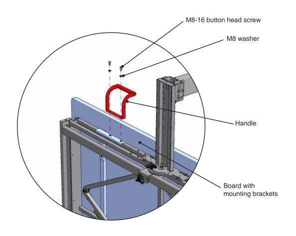
16 - Attach the handles and secure the board using the M8-16 screws and washer through threaded inserts in the Freeframe.
