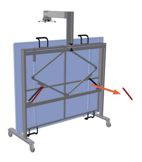
21 - Release the transport brace by undoing the M8-16 button head screws holding the brace to the frame wiuth supplied allen keys.
