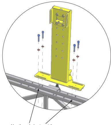
Use these holes to set the projector to the correct offset position for the Hitachi short throw projector.
