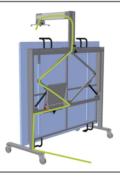
23 - Cables are tied to the frame and scissor system with cable ties. Use the path show in the diagram as a guide in securing loose cables.
