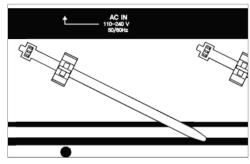
To prevent the power cable from falling/shaking, you may use the cable holder if necessary. SCREW (4x11)
