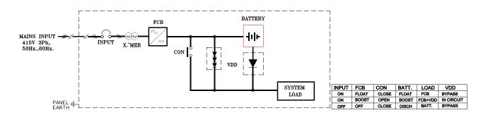
Float and Float Cum Boost Charger - Single Load - Single Battery
