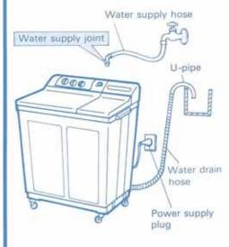
Attach the U-pipe to the end of the Drain Hose and hang onto the brim of a Sink.
