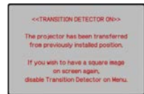
Transition Detector Alarm
