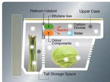
Ethylene gas released by vegetables can spoil their freshness. Platinum catalyst technology has the ability to decompose the ethylene gas and convert it into carbon dioxide gas, delaying spoilage by making vegetables dormant to preserve freshness.
