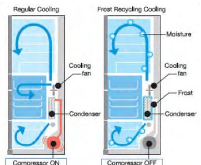
With Regular Cooling systems frost formed on the evaporator simply melts and is discarded.
