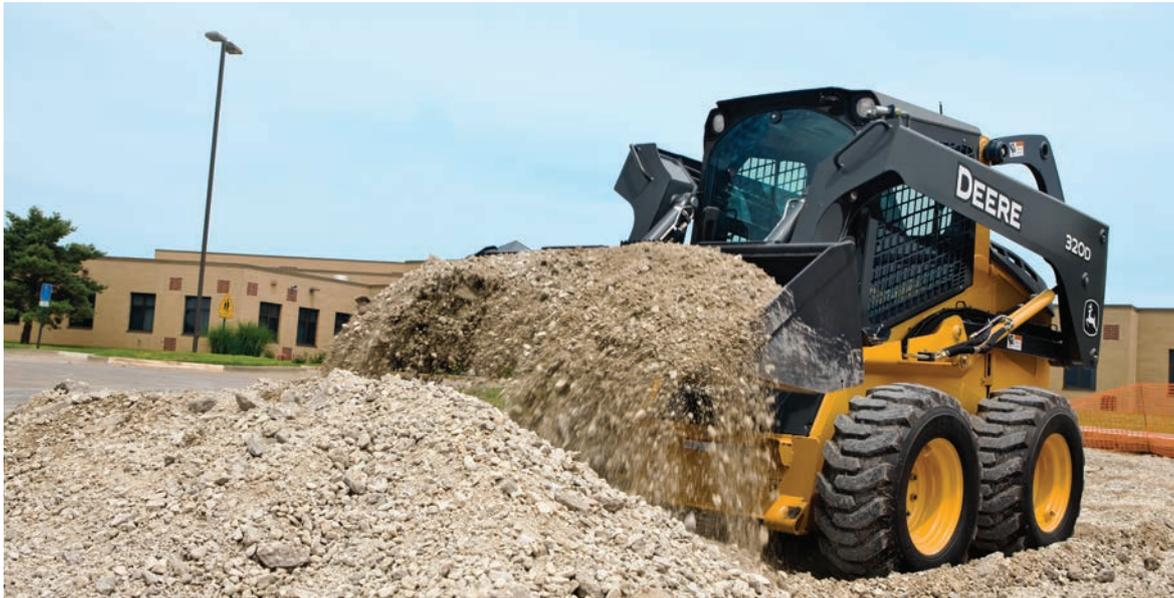
**Left:** Superior axle torque, large standard tyres, and impressive breakout force give D Series Skid Steers the leverage to dig in where others just spin. So they penetrate dirt piles more easily and fill the bucket fuller and faster.
